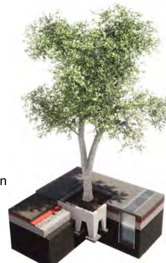
2. Structural Soil Tree Pit 3D view
