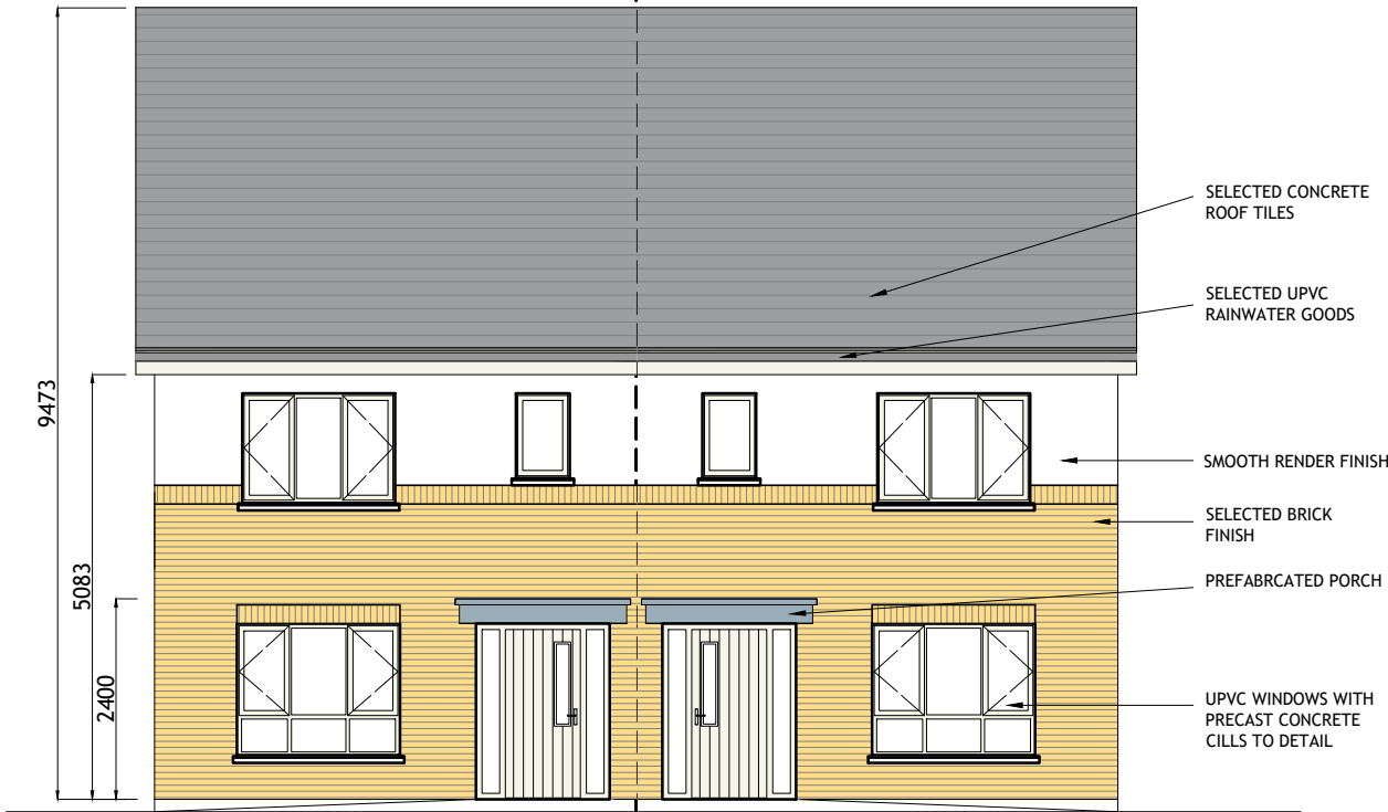
FRONT (ROADSIDE) ELEVATION SCALE 1:100
