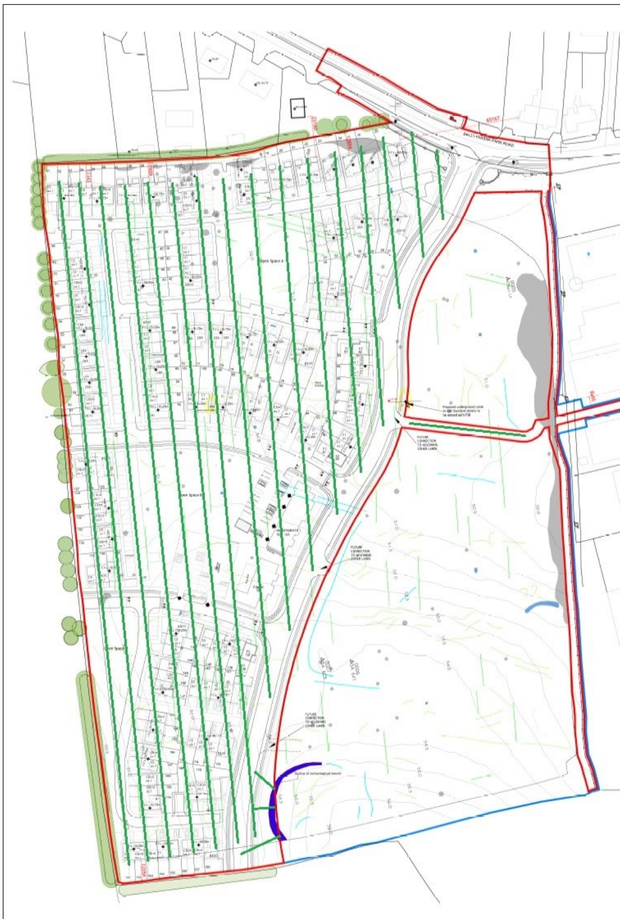
Figure 12: Layout of test trenches, shown in green, to be excavated across the site in advance of development.
